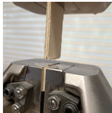
(b) Plywood broken
